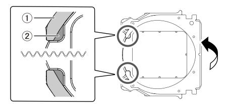
(3) Turn over the adapter so that its top faces up, and then check whether the pin-type workpiece adapter has been mounted on the adapter base without any gaps.
