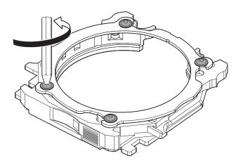
2. Turn the adapter cap in the direction of the arrows to remove it.
