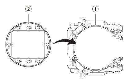
(2) Turn over the loaded adapter, and then align the positions shown in the following figure. Attach the pin-type workpiece adapter so that the protrusions on the adapter base (①) match the positions of the recessed parts on this adapter (②).
