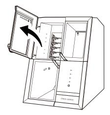
2. Remove the adapter from the adapter magazine.
