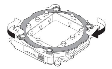
**5.** Temporarily tighten the screws (in four locations) with a torque screwdriver so that their seats come into contact with the adapter cap.
