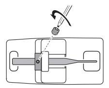
2. Set the milling bur in the ATC magazine.
