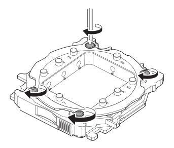
6. Use a torque screwdriver to tighten the screws in four locations in the order shown in the following figure.
