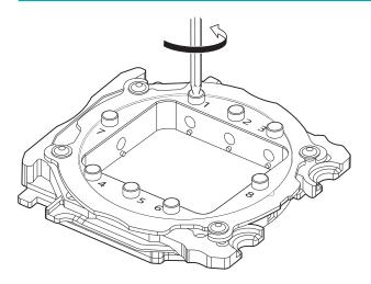
2. Mount the pin-type workpiece on the pin-type workpiece adapter.
