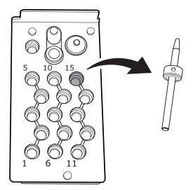
Remove the automatic correction jig from the adapter magazine.Slightly lift up the automatic correction jig, and then pull it out slowly so it does not catch on the stocker.
