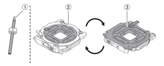
Load the detection pin in the ATC magazine's number 15 position. Insert the detection pin firmly into the ATC magazine.
