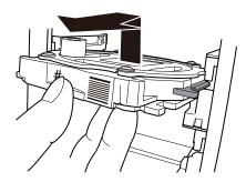
4. Store the detection pin and the automatic correction jig in the bottom storage.
