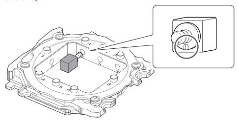
3. Tighten the screw using a torque screwdriver.
