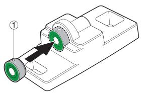
(2) Slide the milling bur through the milling bur holder and determine the proper position.
