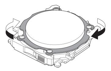
**5.** Temporarily tighten the screws (in four locations) with a torque screwdriver so that their seats come into contact with the adapter cap.
