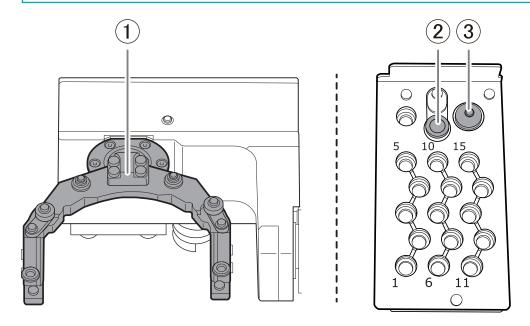
**5.** Wipe the detection pin (①) and the top (②) and bottom (③) of the automatic correction jig clean. Clean the gray parts in the following figure. If any dirt is present in these locations, it may not be possible to perform the correction properly.
