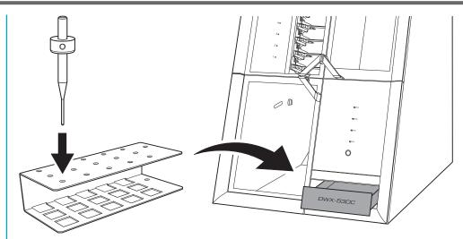
You can store unused milling burs in their cases by standing them in the tool rack with it oriented with its square holes on the top. In this situation, the tool rack will not fit in the bottom storage, so place it next to the machine.
