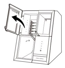
**2.** With its adapter ID facing you, insert the automatic correction jig into the adapter stocker. Insert the adapter slowly.
