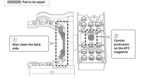
**3** Use the included cloth for care to clean the automatic correction jig and the detection pin. If any dirt is present in these locations, it may not be possible to perform the correction properly.
