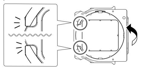
③ Check whether the pin-type workpiece adapter has been mounted on the adapter base without any gaps.
