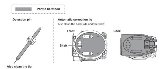
4 Load the detection pin in the ATC magazine's number 15 position.
