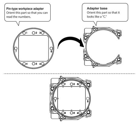
② Turn over the assembly prepared in step ①, and then align it with the positions shown in the figure.
