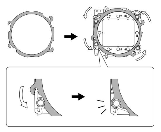
**5** Use a torque screwdriver to tighten the screws in the positions shown in the figure. (4 locations) Tighten the screws until they click.
