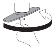
③ Tighten the collet with the wrench while holding the detection pin.
