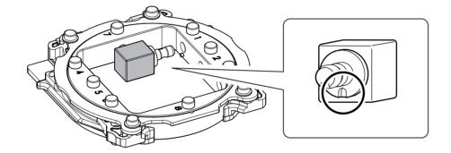
**3** Tighten the screws using a torque screwdriver. Tighten the screws until they click.
