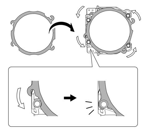
**5** Use a torque screwdriver to tighten the screws in the positions shown in the figure. (4 locations) Tighten the screws until they click.
