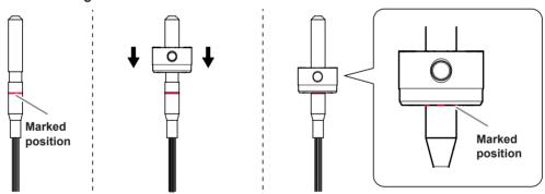
3 Use the mounting screw to fix the milling bur holder in place.
