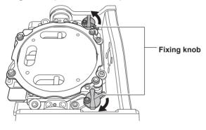
Remove the automatic correction jig.
