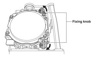
Remove the adapter from the clamp.
