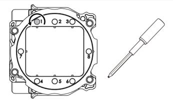
Mount the pin-type workpiece on the pin-type workpiece adapter.
