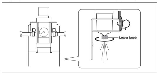
2 After the drain empties, retighten the lower knob.
