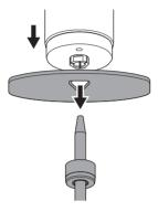
4 Remove the detection pin and the wrench.
